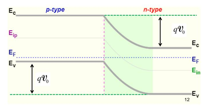
$N_A = 10^{18} \text{cm}^{-3}$  $N_D = 5 \times 10^{15} \text{cm}^{-3}$  The built-in potential  $qV_o$  quantifies the potential energy barrier of the p-n junction. It is determined by the Fermi level position, relative to the intrinsic Fermi level, in the neutral regions.
