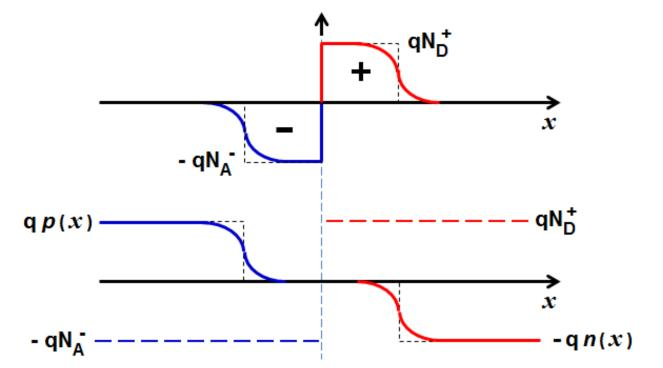
The minority concentration is very minute and it has been neglected in the equilibrium analysis, but minority carriers will be important to understand current injection when a bias voltage is applied.
