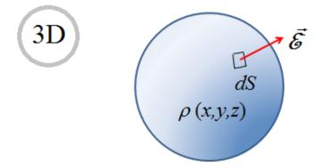
$\vec{\varepsilon} = \text{net charge density enclosed}$   $\vec{\delta} = \text{Electric Field}$   $\iiint_V \frac{\rho}{\varepsilon} \, dV = \bigoplus_S \vec{\varepsilon} \cdot dS = \text{Flux of } \vec{\varepsilon} \text{ through } S$
