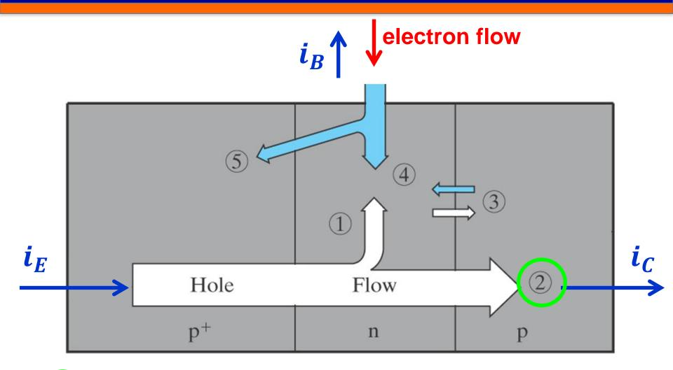
injected holes reaching reverse-biased collector junction
