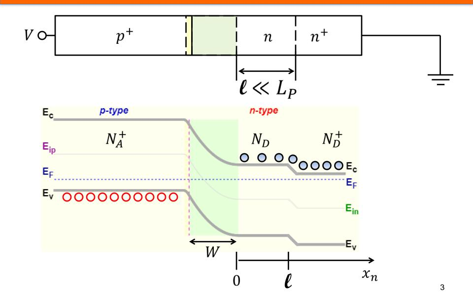
Assume constant cross sectional area. An exact soution of the diffusion equation is obtained from linear combination of exponentials
