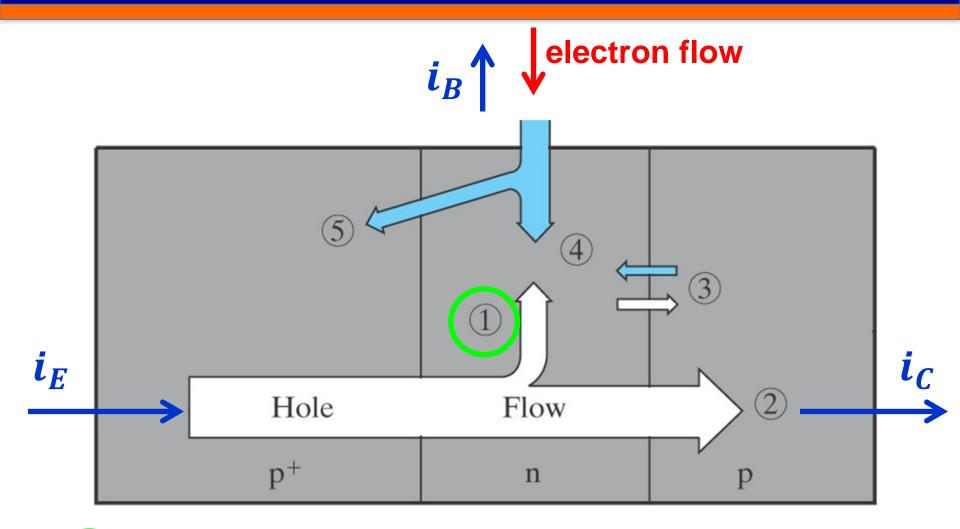
1 injected holes lost to recombination in the base
