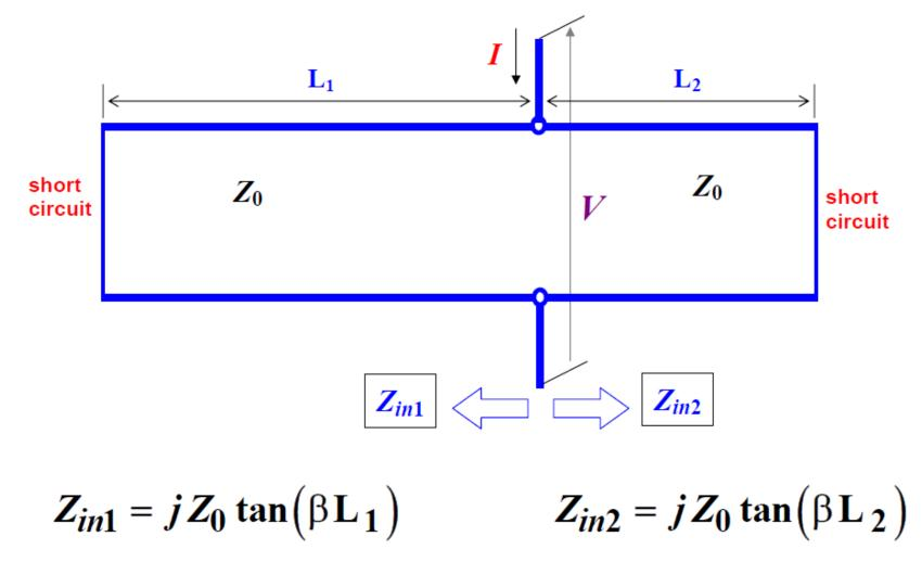
The circuit is resonant if  $L_1$  and  $L_2$  are chosen such that an inductance and a capacitance are realized.
