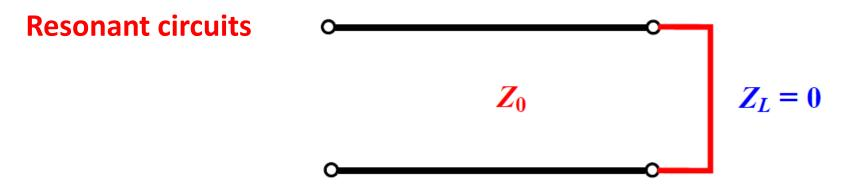
A short-circuited line *stub* is equivalent to an <u>open circuit</u> when the length is an odd multiple of  $\lambda/4$  with resonant frequencies
