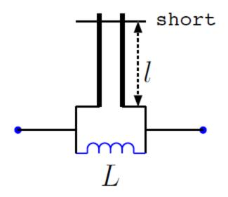
It is possible to realize resonant circuits by using transmission lines as reactive elements. For instance, consider the circuit below realized with lines having the same characteristic impedance:
